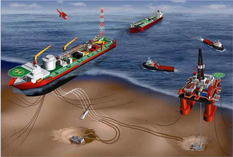
Figure 2.3: Different types of floaters used in the development of the Terra Nova field on the Grand Banks, Lever et al. [5].
