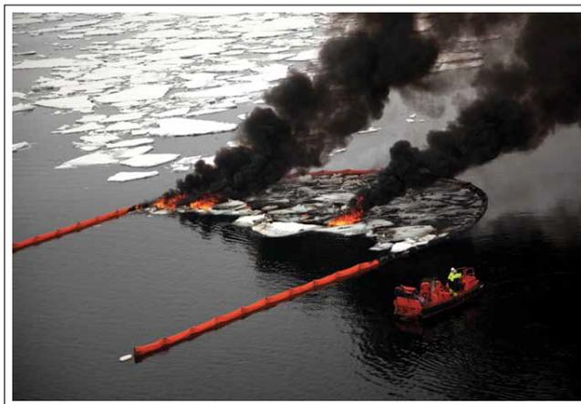
**Figure 8.5:** Controlled in-situ burning for JIP Project. *Source:* [SINTEF](#)
