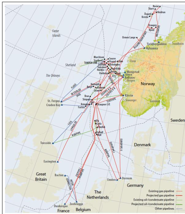
**Figure 5.6:** Existing and projected pipelines on the Norwegian Continental Shelf.
