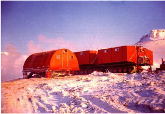
**Fig. 7.** Tracked camp for Big Indian Drilling Rig 3. On Ellef Ringnes Island near Kristoffer Bay. The rig drilled shallow holes to determine the depth of the permafrost. The depth varied from 200 m to 400 m.
