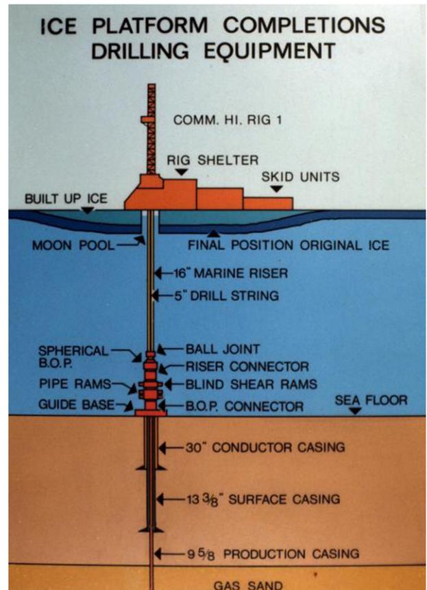
Fig. 28. Section of ice platform and drill assembly.
