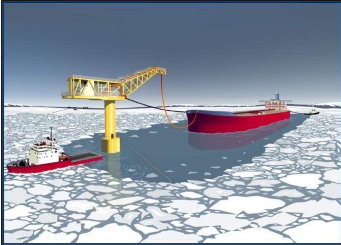
The export tanker moors up to the TLU and an ice breaker tug fitted with the Aquamaster propulsion system positions itself updrift from the TLU. By spreading the Aquamasters at approximately 80 deg. the tug maintains position and the propeller wash creates a wide swath of open water, the technique has been used and proven in Vityaz operations.
