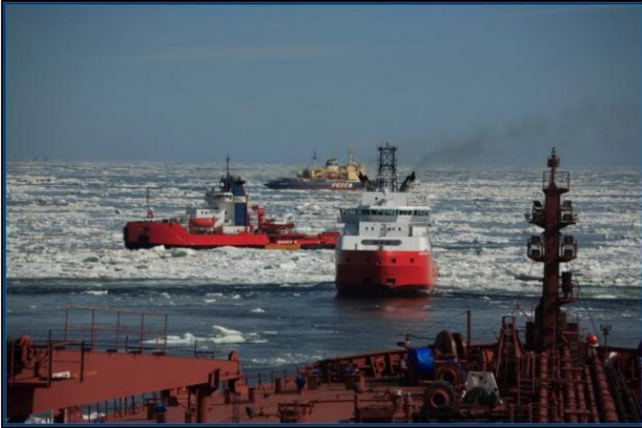
With the help of an Ice Management Team crude oil production and exports continued until ice reached 30 cm of thickness or was no longer manageable. The platform supply vessels were utilized for ice management duty. Equipped with Aquamasters the boats could keep station while providing open water work environment for the FSO and the SALM laydown operations by angling out the Aquamasters, using high power and blasting the ice away. For this to be effective the ice had to be pre-broken.
