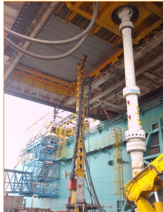
BOP in moonpool on RS and RollSafe deck installed
